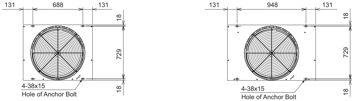
Fig. 5.1 Position of Anchor Bolts
